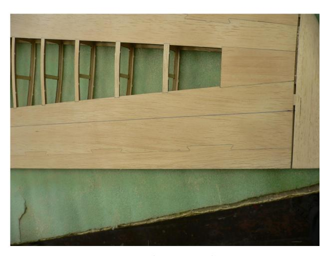
Warning: ailerons cut and glue the balsą strips of sand at an angle of 45 degrees
