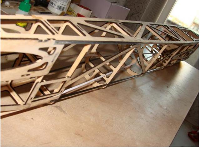
WARNING: Before applying fuzelage balza, all parts assembled PVA glue
